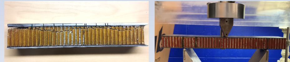
Fracture tests on honeycomb sandwich
